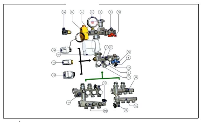
three-way mixing valve, thermostatically operated or motor-driven (without having to replace the insert) 1a. thermostatic head with remote immersion probe, adjustment field 30÷50°C 1b. electro-thermal head 24 VAC proportional 0-10 V 1c. axial servo-motor 24 VAC proportional 0-10 V
